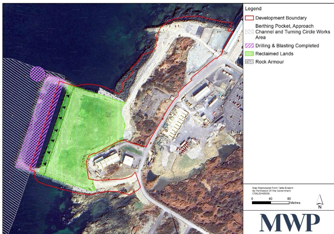
Figure 2-7: Map indicating the development works area, including the reclamation area, the blasting and dredging areas, the berm construction areas and rock armour placed undertaken between Jan 2023 and May 2024.
