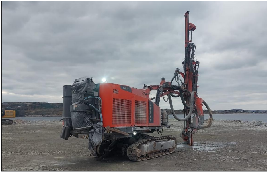
Figure 2-19: Drilling Rig used to drill the blasting holes.
